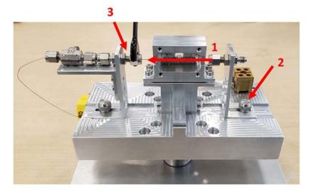
4) Push the thermocouple close to, but not into the sample, and not into the direct beam. Then tighten the nut until the thermocouple can't be easily pulled out, and not much more than that.
