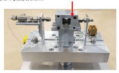
6) Transfer the assembly into the endstation: Take care not to bump the collimator, beamstop, and especially the detector!!!
