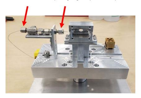
2) Nut and ferrule installed over capillary. Carefully tighten the nut a little at a time, until the capillary can't be pulled out. Then go a little beyond that... not much more than that, maybe a 1/16th of a turn.
