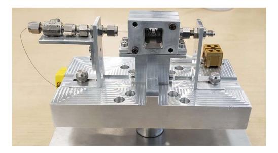
The furnace is very flexible! We have different sets of fittings, ferrules, and thermocouples. It can handle capillaries as large as 3.0 mm OD. The specific conditions of the experiment should be bench tested before attempting to measure with beam.
