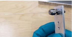
3) Guide the capillary through the heating coil (1), over the thermocouple, and into the ferrule. Finger tighten the thumbscrew for the L bracket (2), then tighten the nut (3) until the capillary can't be pulled out, and not much more than that.
