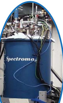
Superconducting magnet: T: 2 ~ 325K H: 0 ~ 7 Tesla
