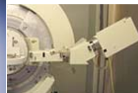
Graphite analyzer (diffracted beam monochromator) rejects fluorescence & K\beta ( K\alpha_2 remains)
