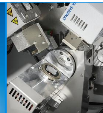
Figure 2 Measurement geometry for residual stress measurements in the D6 PHASER. Shown is the optional phi attachment which enables biaxial stress measurements.
