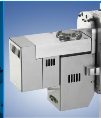
Figure 2 Universal stage equipped with phi attachment
