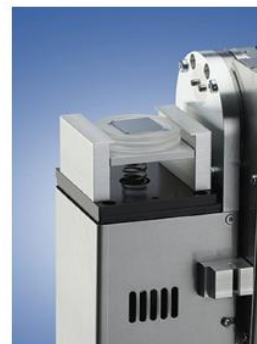
Figure 1 Universal stage with spring sample holder
