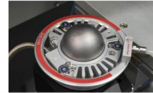
The Anton Paar domed heating stage (DHS1100) can be used to heat flat plate samples from ambient temperature to 1100 °C in a variety of inert gas atmospheres or under vacuum.
