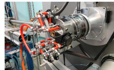
A Stoe capillary furnace can heat capillaries up to 1770K. Quartz capillaries can be used up to 1370 K, above which sapphire capillaries must be used. Users must supply their own sapphire capillaries.
