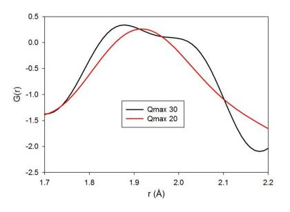
Neutron PDFs of Sr<sub>2</sub>FeMnO<sub>5</sub> created with 2 different Q<sub>max</sub> values.
