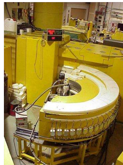
The BT-1 diffractometer at the NIST NCNR. It has 32 detectors that only need to rotate 5 degrees.
