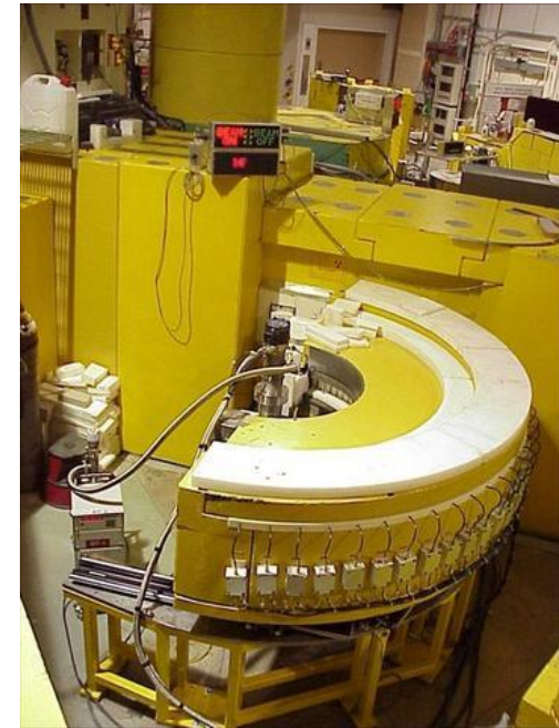
The BT-1 diffractometer at the NIST NCNR. It has 32 detectors that only need to rotate 5 degrees.
